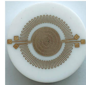
Aerosol Jet printed strain sensor on ceramic
